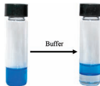
Figure 3. Photographs of buffer-out phase separation behavior of the 1,4-dioxane + MOBS + water system. The color is due to disperse blue 14 dyestuff.
